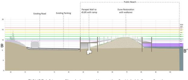
FIGURE A-14. Circuit Avenue Alternative 2 – Hybrid, Cross-Section
