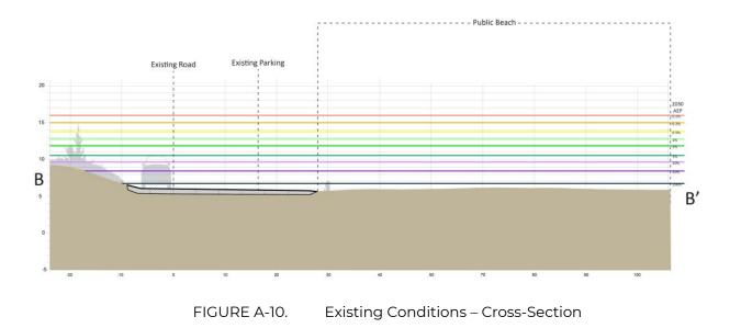
The colored, horizontal lines represent different flood probabilities for 2030 using the MC-FRM.
