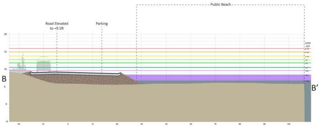
FIGURE A-12. Circuit Avenue Alternative 1 – Gray, Cross-Section
